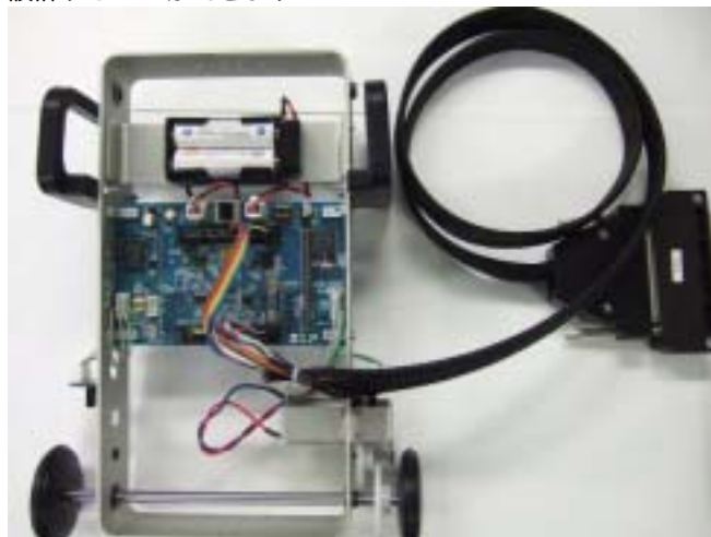
Fig.1 External view of the wheeled inverted pendulum
