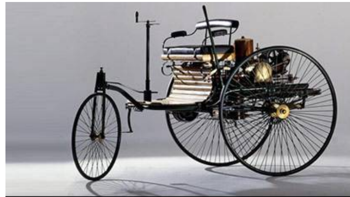
Fig.1 1886 Benz "Patent Motor Car" First high-speed single-cylinder four-stroke engine.
